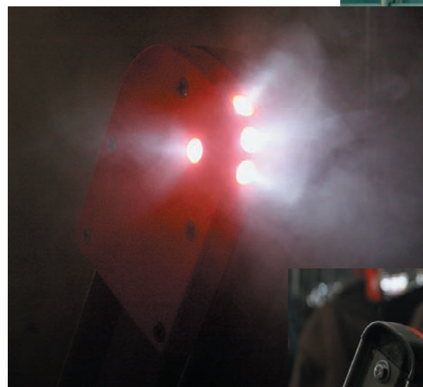
Four hi-intensity LED's rated at more than 25,000 mcd each. When the ladder is properly deployed against a window, one LED is directed downward towards the floor, one straight ahead and another upward towards the ceiling as well as one facing the side.
