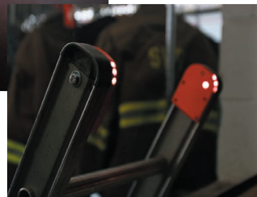
Four hi-intensity LED's rated at more than 25,000 mcd each. When the ladder is properly deployed against a window, one LED is directed downward towards the floor, one straight ahead and another upward towards the ceiling as well as one facing the side.
